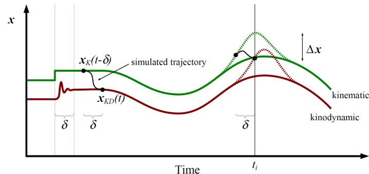
This plot illustrates how we modify a kinematic trajectory to create a kinodynamic trajectory satisfying the constraint that the original kinematic state be produced at time  $t_i$ .
