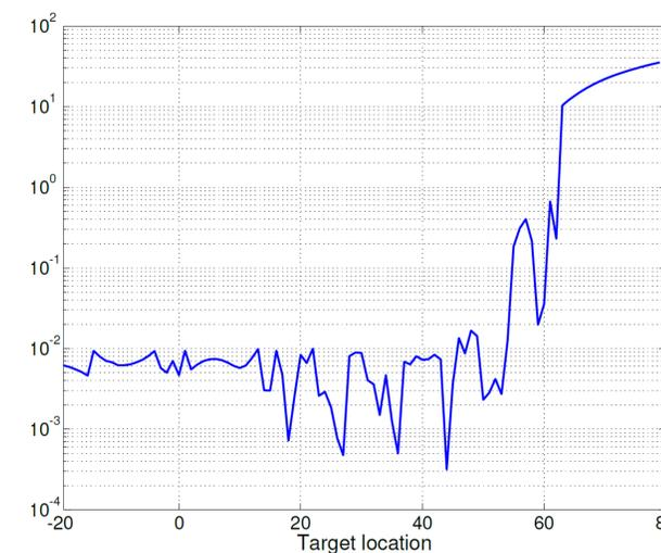
IKD error in cm after 6 iterations for varying target locations in the punch scenario. The error consistently falls to less than 0.1 mm after 6 iterations, except when the target is out of reach.
