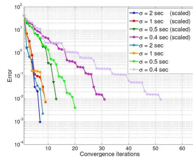
IKD convergence rates for the punch scenario using a bell shaped correction function with different temporal widths, with end effector error measured in cm, and error threshold  $10^{-2}$  cm. The IKD convergence can be slower when a small temporal width is used, but is improved by damping the correction adjustment by 0.8, as shown by the trajectories denoted (scaled).
