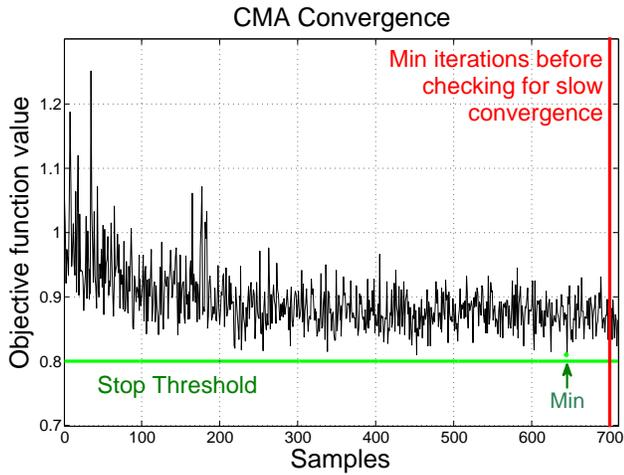
**Figure 4:** A plot showing objective function values for all samples computed during a CMA optimization, along with the stop threshold value. In this case the minimum of 700 samples was passed, after which a test for slow convergence terminated the optimization.
