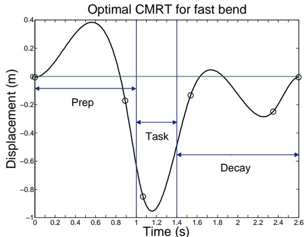
**Figure 3:** Example CMRT trajectory for the fast bending motion.
