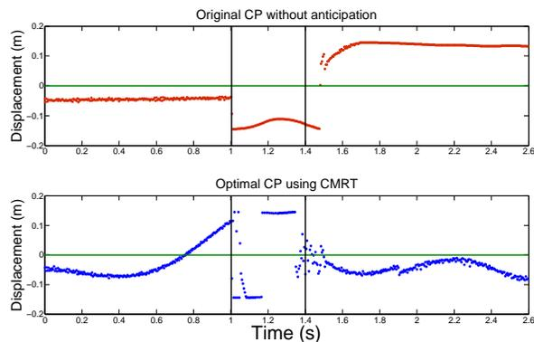
**Figure 2:** Example CP trajectory optimization for the fast bending motion. The top and the bottom plots show the CP before and after applying CMRT.
